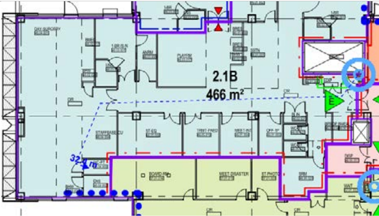
Fire hydrant coverage departure in compartment 2.1B
