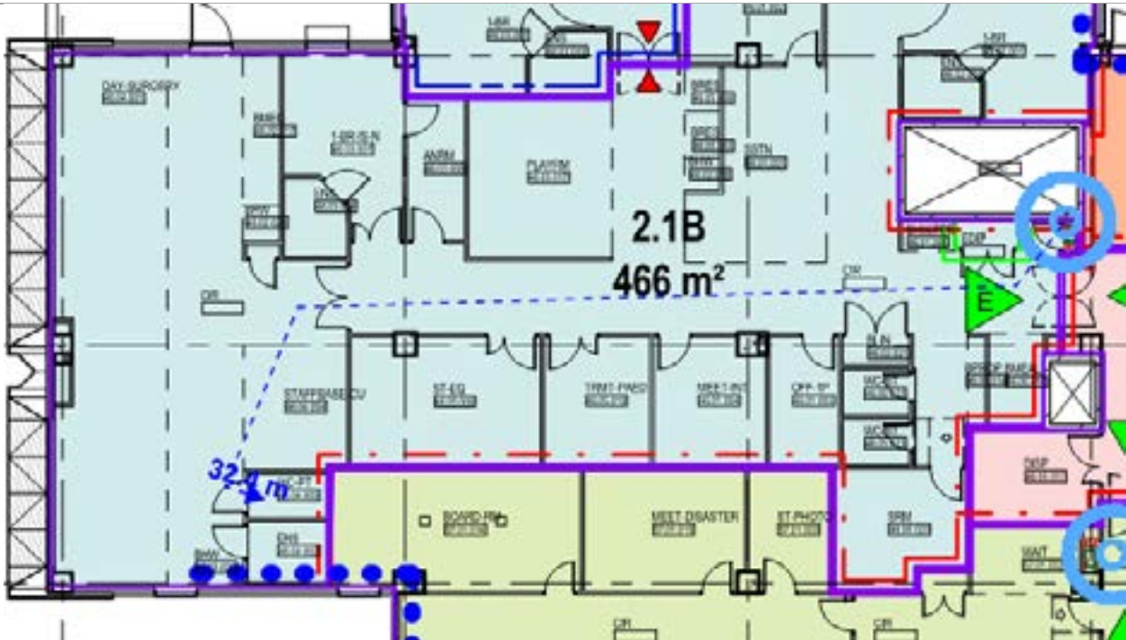
Fire hydrant coverage departure in compartment 2.1B
