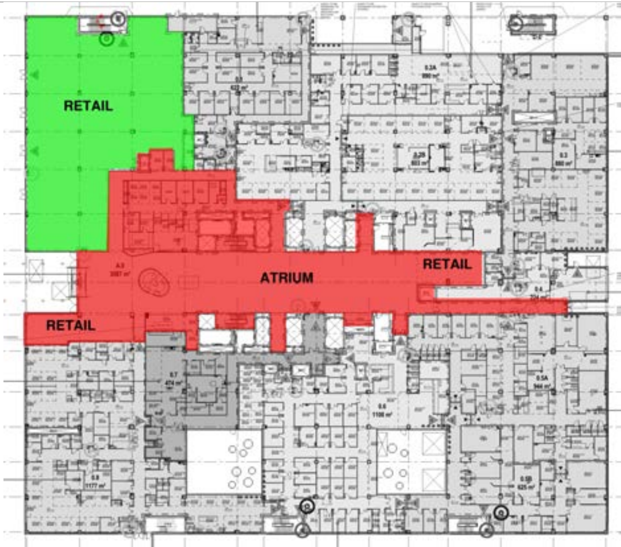
Smoke compartments on Ground Floor
