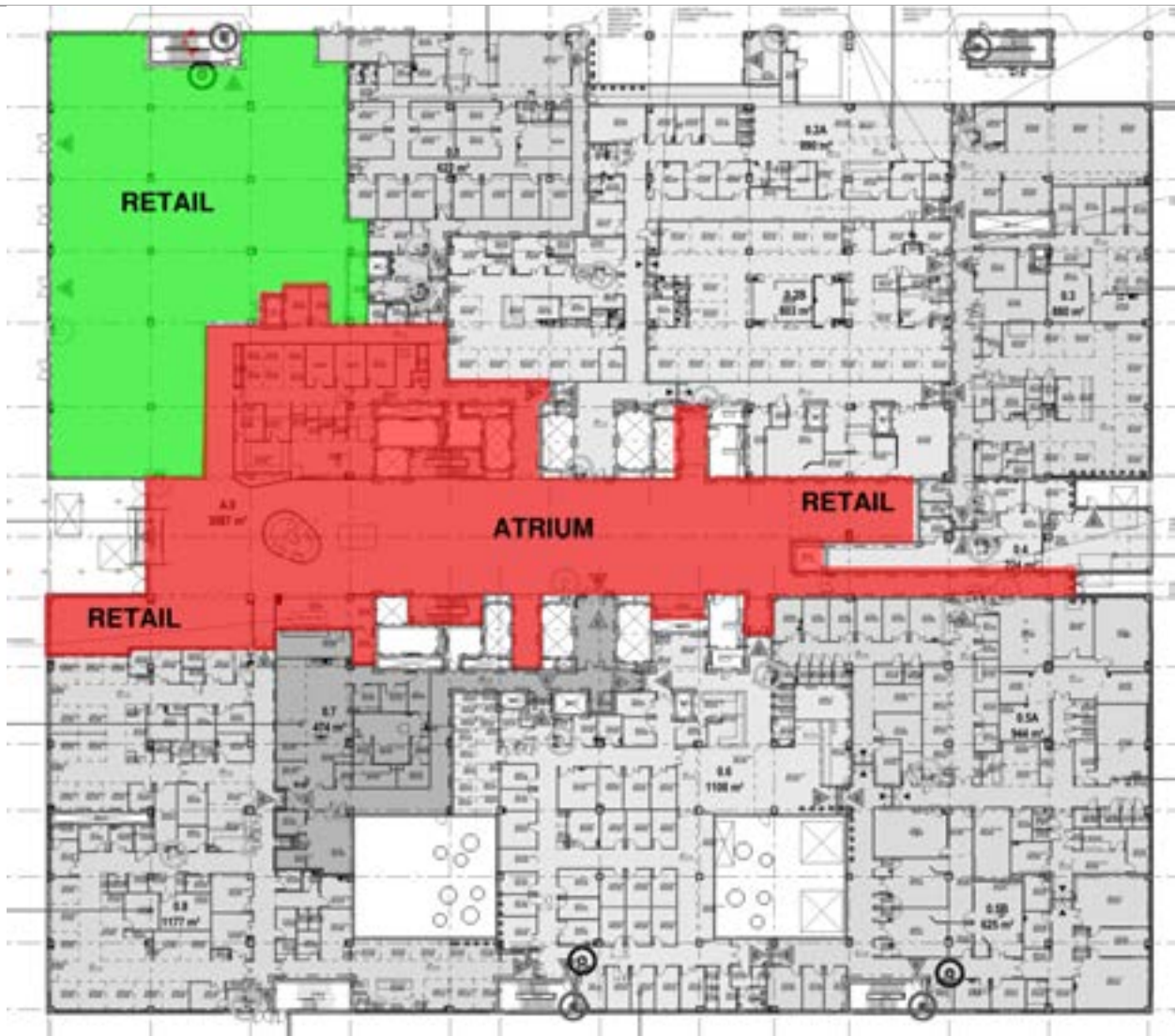
Smoke compartments on Ground Floor
